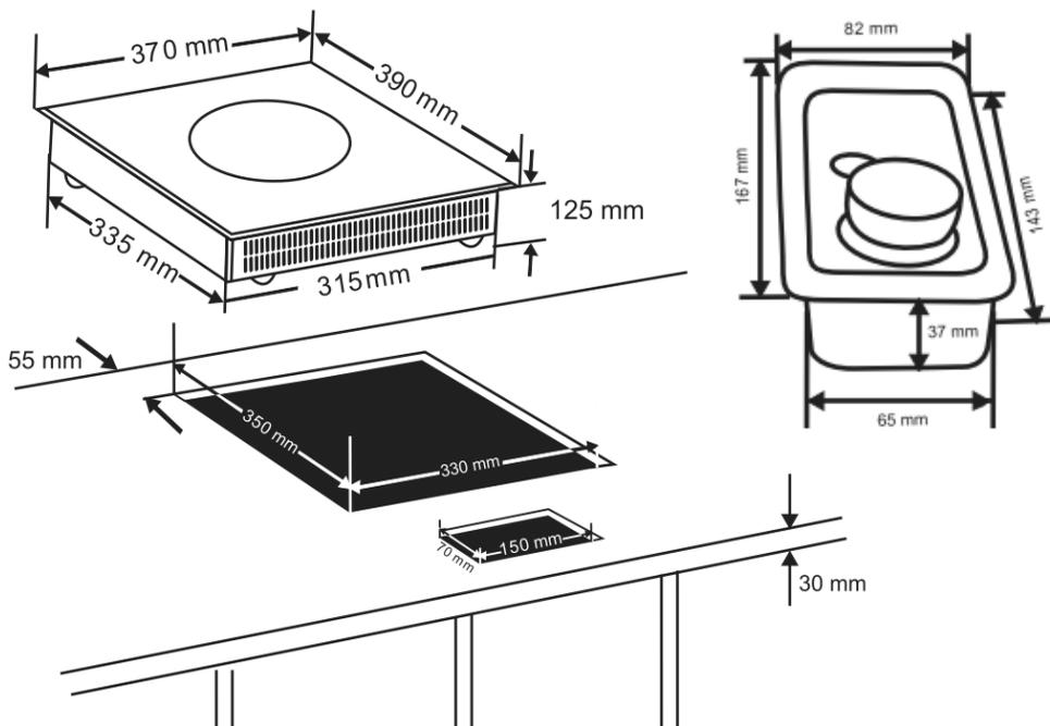
4. Provide sufficient ventilation around the device and make sure that the ventilation holes are not blocked.
