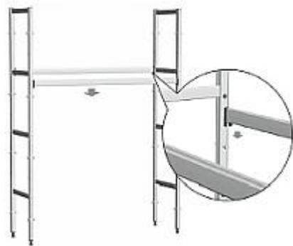
1. Insert the screws connecting bars into suitable bores in both side elements.
