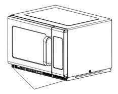
• Loosen the screws on the right side at the filter and remove the filter.
