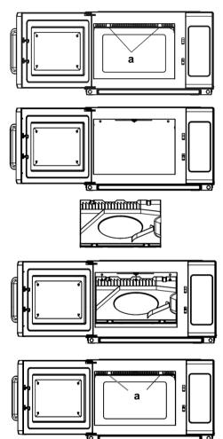
Set the upper splash guard in the initial position. Remember to insert 3 hooks into the holes at the rear of the device.
