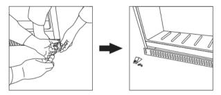
7. Unscrew hinge 4 from the bottom door attachment.
