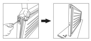
8. Unscrew hinge 3 from the bottom door attachment.
