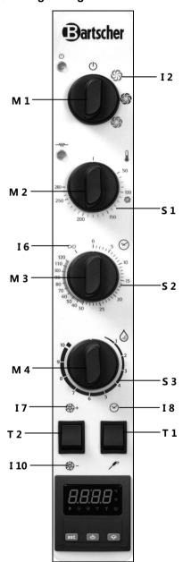
To set cooking/baking with the use of RECIRCULATED AIR, turn the M 1 function dial clockwise to the position I 2.
