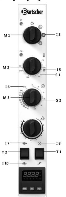
To set cooking/baking with the use of **STEAM**, turn the function dial **M 1** clockwise to the position **I 3**.
