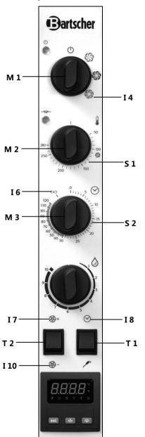
To set **STEAM CONVECTION cooking** (cooking/baking with the use of recirculated air/steam) turn the function dial **M 1** clockwise to the position **I 4**.
