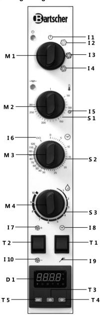
After selecting the desired cooking/baking mode and setting the function dial in one of the positions I 2 – I 3 – I 4, set the temperature.
