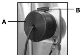
To connect the core temperature sensor take out the plug **A** (image on the left) from the opening at the top left side of the oven, press and hold the red detent **B** and insert the core temperature sensor **C** into the opening provided.
