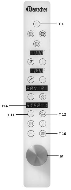
To select a stored program, use **T 12** button and select the desired program number by turning **M** dial clock or counter-clockwise. Confirm the selection by pressing **T 12** button when the desired program **"PRG 04"** is displayed.
