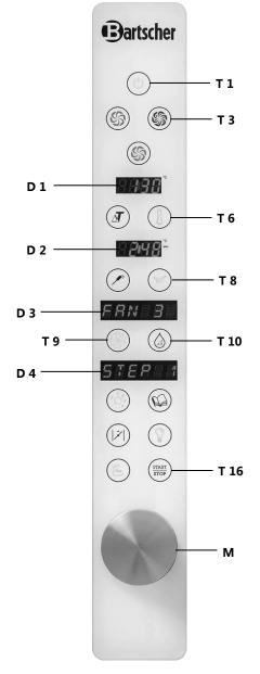
To turn the device on, press the button **T1**. The function buttons **T 2 – T 3 - T 4** will flash, and the device is ready to accept function settings. The LED display **D 4** will read "MANUAL".
