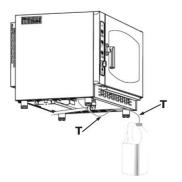
The supply hose for cleaning agents is permanently connected to the pump in the lower part of the device.
