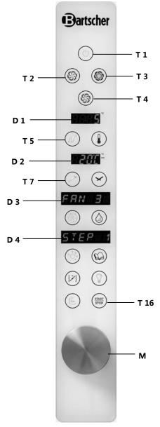
To turn the device on, press the button T1. The function buttons T 2 - T 3 - T 4 will flash, and the device is ready to accept function settings. The LED display D 4 will read "MANUAL".
