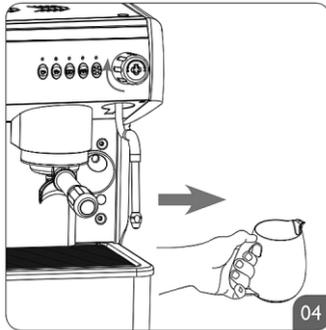
4. When the milk reaches the required temperature, close the steam tap and remove the container.
