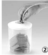
Connect the lid with the vacuum packing machine pump via the hose.
