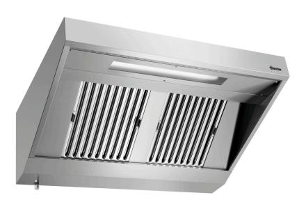
With its integrated motor and 2 filters, the extractor hood offers high suction power over a large surface area. The stainless steel design with a motor power of 145 watts and a maximum air throughput of 1475 m<sup>3</sup>/h is intended for wall mounting and fitted with LED lighting.
