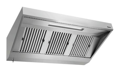
With its integrated motor and 3 filters, the extractor hood offers high suction power over a large surface area. The stainless steel design with a motor power of 145 watts and a maximum air throughput of 1928 m<sup>3</sup>/h is intended for wall mounting and fitted with LED lighting.
