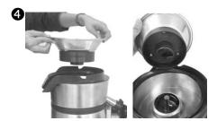
Tilt the sieve (10) position it above the juice bowl (14) and place it on the motor drive (8) by turning slightly to interlock the pin at the motor base with the groove at the bottom of the sieve (10).
