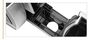
This model is supplied with a "chute hole" in the housing. This offers you the option of disposing the coffee grounds directly through the ejection chute into a waste bin. The grounds container has a capacity for 35 cups.
